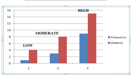
FIG 14: GRAPH ON FREQUENCY V/S DISTANCE "WHEN THE FREQUENCY OF RFID READER IS HIGH THEN CAPABILITY TO ACCESS DATA FROM A RFID TAG AT A LONGER DISTANCE IS POSSIBLE"
