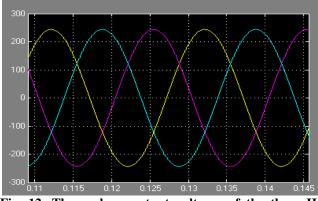
Fig. 12. Three phase output voltages of the three H6 topologies.
