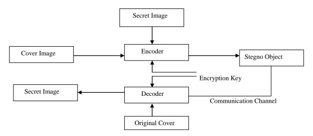
Fig. 2 Generic Process of Encoding and Decoding
