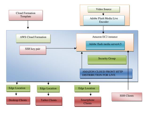
Figure 2. Cloud Front Live streaming architecture
