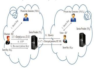
Fig3. Identity based data storage supporting inter domain Query.
