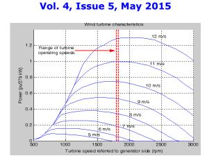
Fig. 4. Turbine power characteristics
