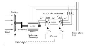
Fig.7. Variable-speed wind turbine with DFIG
