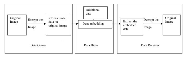
Fig: 3 Architecture for Encrypting and Embedding image
