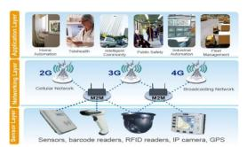
Figure 3.IOT architecture with example devices in each layer [10]
